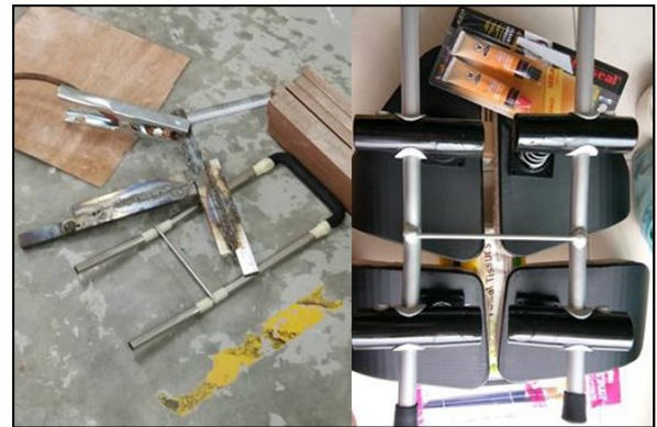
Figure 10. The fabrication of metal structure, and the installation of the spinal support adjuster.
