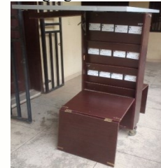
Fig. 5. The kiosk showing the arrangement of the charging Outlets
