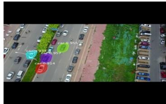
Fig. 10. Result of Mask R-CNN-Adam Optimizer
