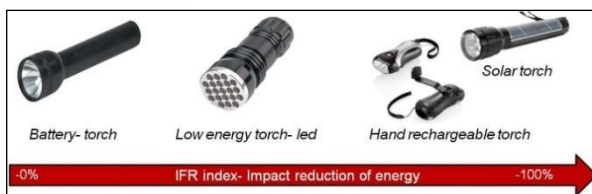
Figure 3- An example of IFR Redesign on a battery torch. IFR thinking forces to conceive solutions not using any pollutant sources as the hand rechargeable or solar torches
