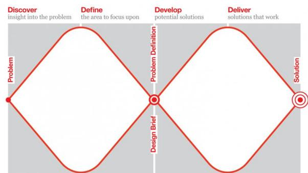
**Fig. 1** Double diamond model of the innovation process (Design Council, 2007).
