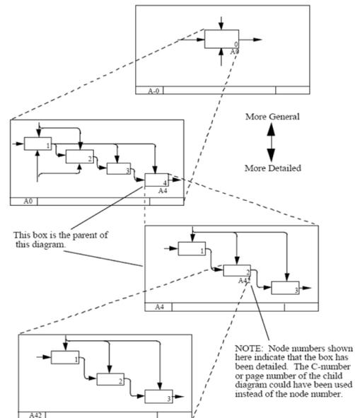
**Fig. 6** IDEF0 decomposition model structure (KBSI, 2005).
