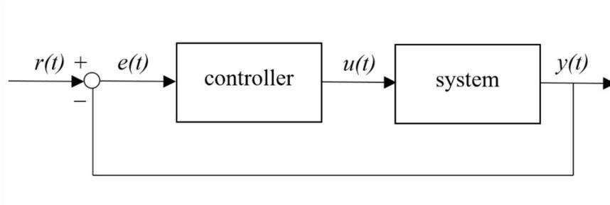
**Fig. 4** Block diagram of feedback control theory
