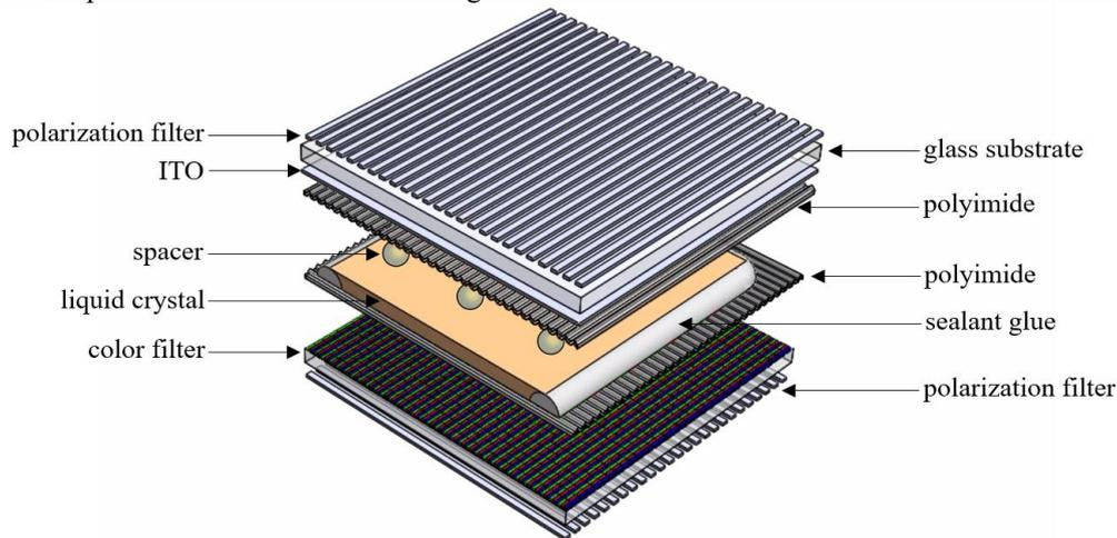
**Fig. 1** Exploded View Diagram for LCD panel
