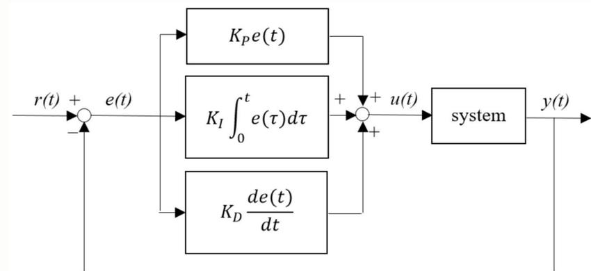
**Fig. 5** Block diagram of PID control theory
