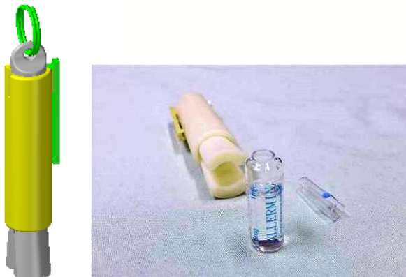
Fig. 2 The new ampoule opener design and prototype.
