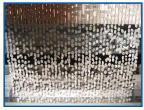
**Fig. 3** The grains of rice fell down in a curtain-like waterfall manner from the groove of the color sorter.
