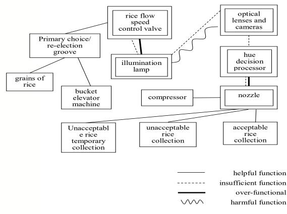
Fig.5 Analysis of functional attributes of the color sorter components.
