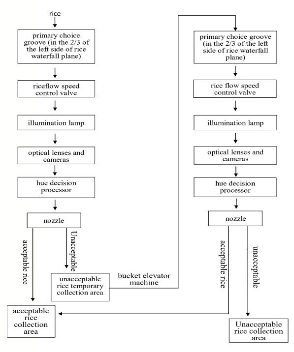
Fig. 4 Flow diagram for rice quality evaluation via color sorting machine.
